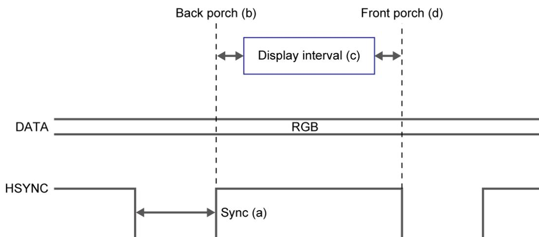
Figure 3-23 VGA horizontal timing specification
