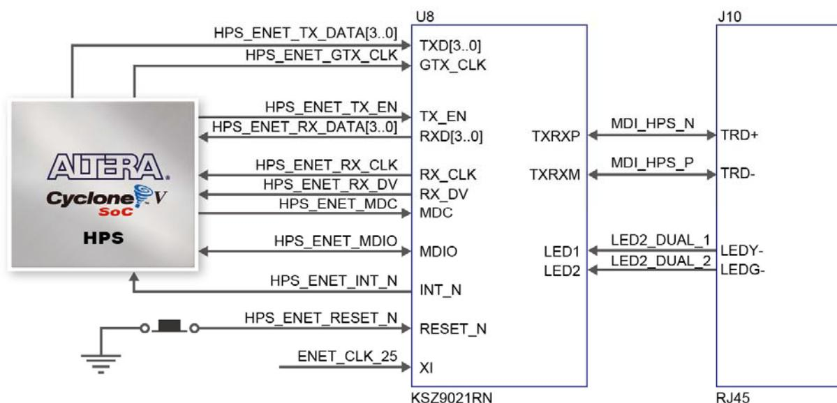
**Figure 3-32 Connections between the HPS and Gigabit Ethernet**
