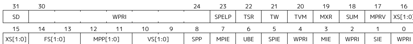
Figure 7. Machine-mode status ( mstatus ) register for RV32
