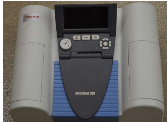
Figure 1 – Top view of a Spectronic 200 spectrophotometer.
