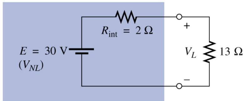
$$P_{R_{int}} = \frac{V_{R_{int}}^2}{R_{int}} = \frac{(30\text{ V} - 26\text{ V})^2}{2\ \Omega}$$
