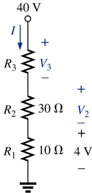
$$V_2 = 3 \cdot 4\ \text{V} = 12\ \text{V}$$
