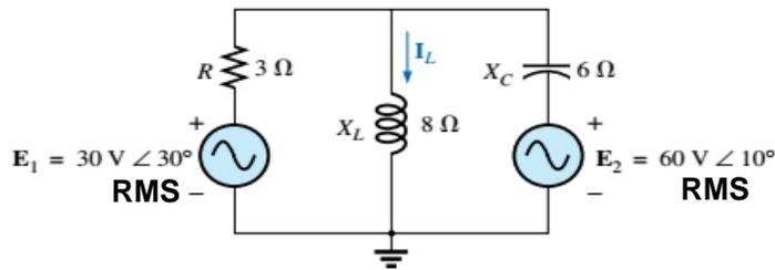
① REDRAW THE NETWORK W/ THE FIRST SOURCE ENERGIZED + THE SECOND SOURCE DEACTED
