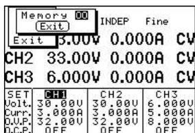
Example : The current setting store address of instrument is at “00”. Press [SHIFT][STORE] getting into item selection picture, using the knob to set the cursor to [STORE], then press [ENTER] and input [0][0][ENTER] directly to complete storing setting.
