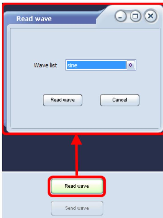
2. On the **Read wave** pop-up, select the desired waveform from the **Wave List**. This list will include the names of all the built-in arbitrary and saved waveforms.
