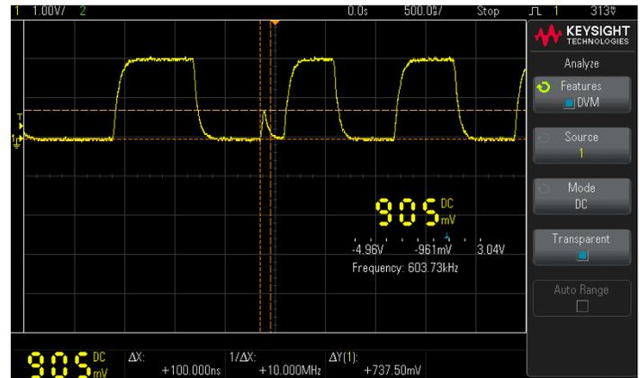
The DVM makes accurate RMS measurements when the signal frequency is between 20 Hz and 100 kHz.
