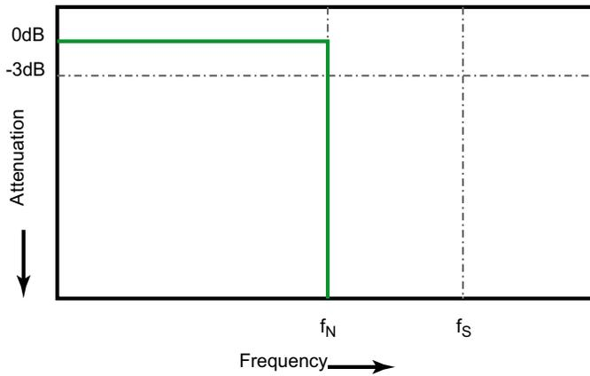
**Figure 4** Theoretical Brick-Wall Frequency Response
