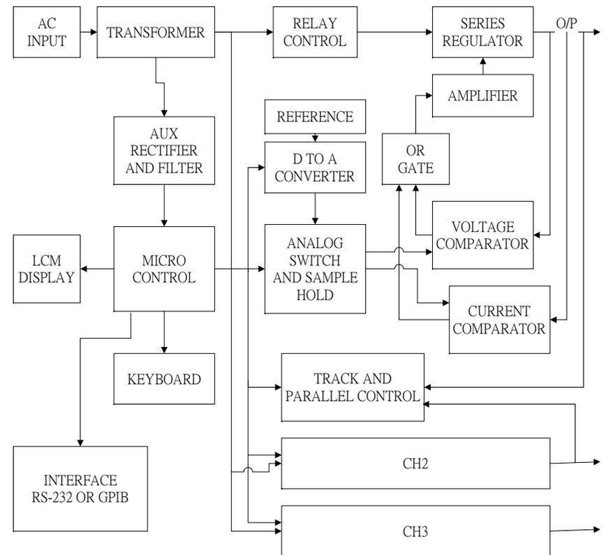
The graph above is the system diagram of PST-SERIES, Which consists of Micro Processor Unit (MPU), Digital to Analog Converter (DAC), Analog Switch Circuit, Reference Voltage Circuit, Driver Circuit, Control Circuit, Track/Parallel Circuit, Comparator, and etc.
