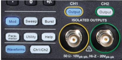
These Front Panel buttons control major functional areas of the software. They appear white when inactive, unlike the navigation and selection controls, which are black.
