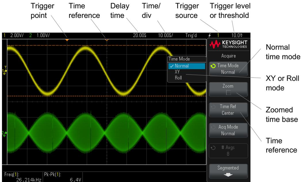
The time reference is indicated at the top of the display grid by a small hollow triangle (▽). Turning the Horizontal scale knob expands or contracts the waveform about the time reference point (▽).
