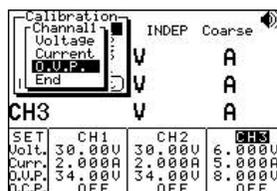
Note: Now, the calibrated data of channel 1 has not yet been stored. If the calibration is aimed at channel 1 only, can set the cursor to [Save] by using the knob and press [ENTER] to finish the procedure with storing.
