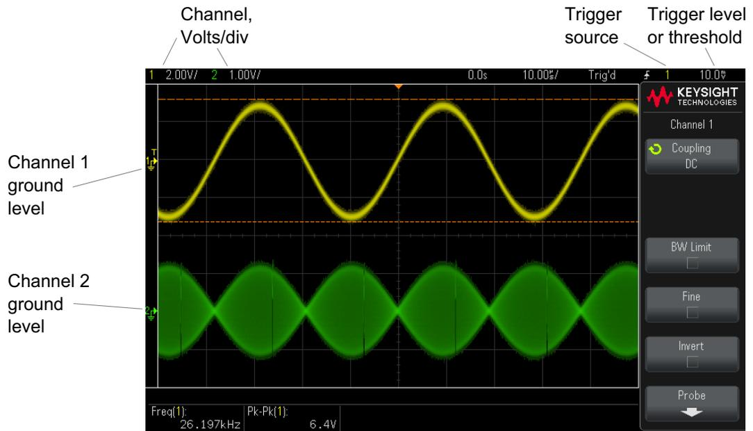
The ground level of the signal for each displayed analog channel is identified by the position of the
