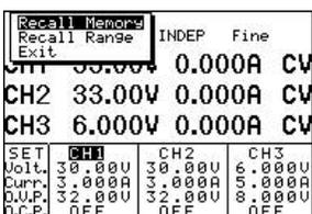
Example: Recall the storing address “00” to the current setting status of instrument. Press [SHIFT][RECALL] getting into item selection picture, using the knob to set the cursor to Recall Memory. Press [ENTER] and input [0][0][ENTER] to complete recalling setting.
