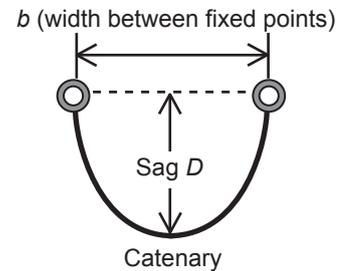
When  $a = 0.846$  and  $b = 2$ , find the rope sag  $D$  and the rope length  $L$ .
