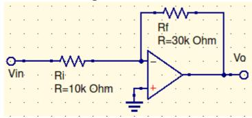
Assume that the op-amp slew rate is  $0.5V/\mu s$ . Calculate the rise time  $T_{SR}$  due to the slew rate when the input is a pulse that changes from zero to each of the following values:
