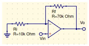
Assume that the op-amp slew rate is  $0.6V/\mu s$ . Calculate the rise time  $T_{SR}$  due to the slew rate when the input is a pulse that changes from zero to the following values:
