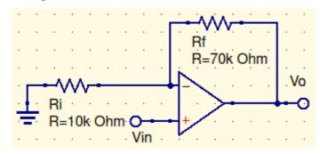
If the unity-gain frequency of the op amp is 1.6MHz, determine the closed loop 3-dB bandwidth.
