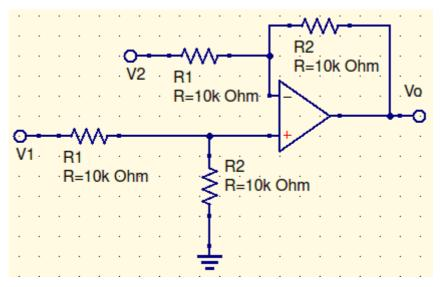
If the unity-gain frequency of the op-amp is 1MHz, determine the closed-loop 3-dB bandwidth.
