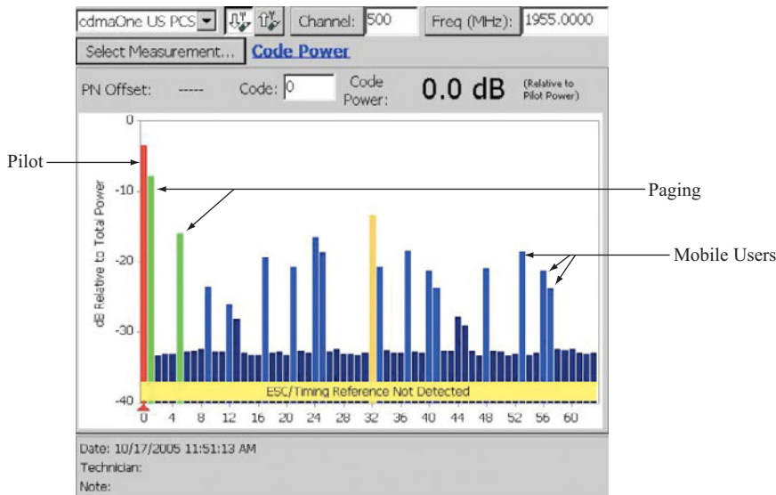
FIGURE 10-16 Display photo from Tektronix YBT250, showing Walsh codes. Walsh code 0 (red) is the Pilot, codes 1–6 (green) are paging, code 32 (yellow) is synchronization, light blue codes are actual mobile users, and dark blue codes are Walsh codes not in use. (Note: This measurement was made over the air; “ESC/Timing Reference Not Detected” indicates that the YBT250 is not physically connected to a base station.)
