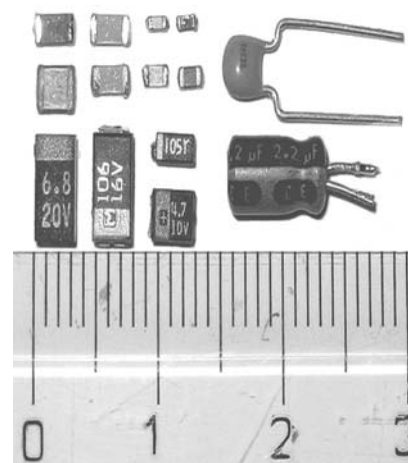
FIG. 1-12. Chip and ceramic capacitors. (Courtesy of Wikipedia)
