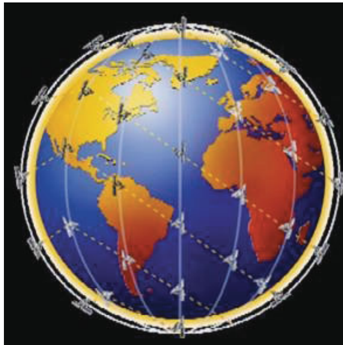
FIGURE 13-19 A picture of the Iridium LEO satellite constellation. (Courtesy of Iridium Satellite LLC.)
