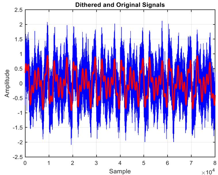
Digitally generated gaussian random noise with a  $\sigma$  of .35 CV is added to the input signal
