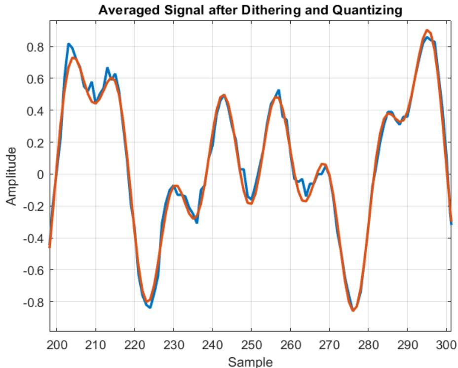
The dithering and averaging has allowed us to recover the original signal even though it was small compared to a quantization level
