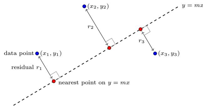
Figure 3: A residual is the perpendicular distance between observed data and the line of fit.
